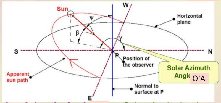
Solar Azimuth Angle O'A : Solar Angle in degrees along the horizon east or west of North.
