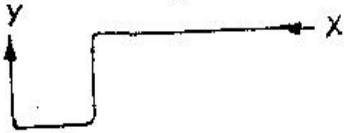
(f) Combination of U and line flow pattern
