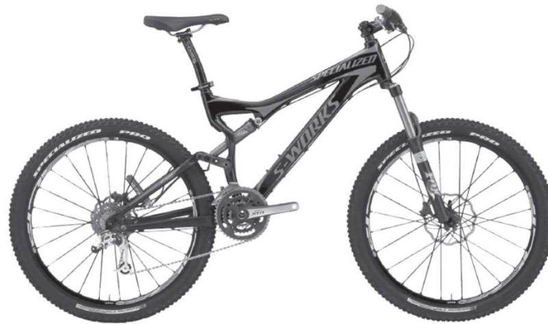
Figure 2.2.1 One of Specialized's existing mountain bikes with a suspension fork.
