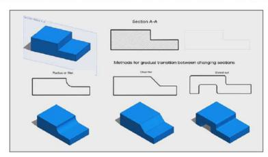
Hollow sections complicate die design and plastic flow. It is desirable to use extruded cross sections that are not hollow yet satisfy functional requirements
