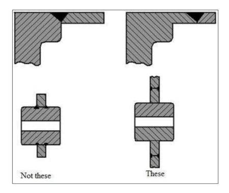
The joint should be designed so that it requires minimal edge preparation. For this, one should use slip or lap joints in welded assemblies to avoid the cost of close edge preparation and to simplify fit-up problems.
