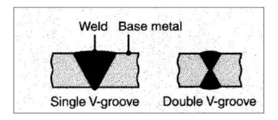
The designer should be aware of poor and good fit-up of parts at the weld joint. It is essential not only for welding speed but also for minimizing distortion of the finished weldment.
