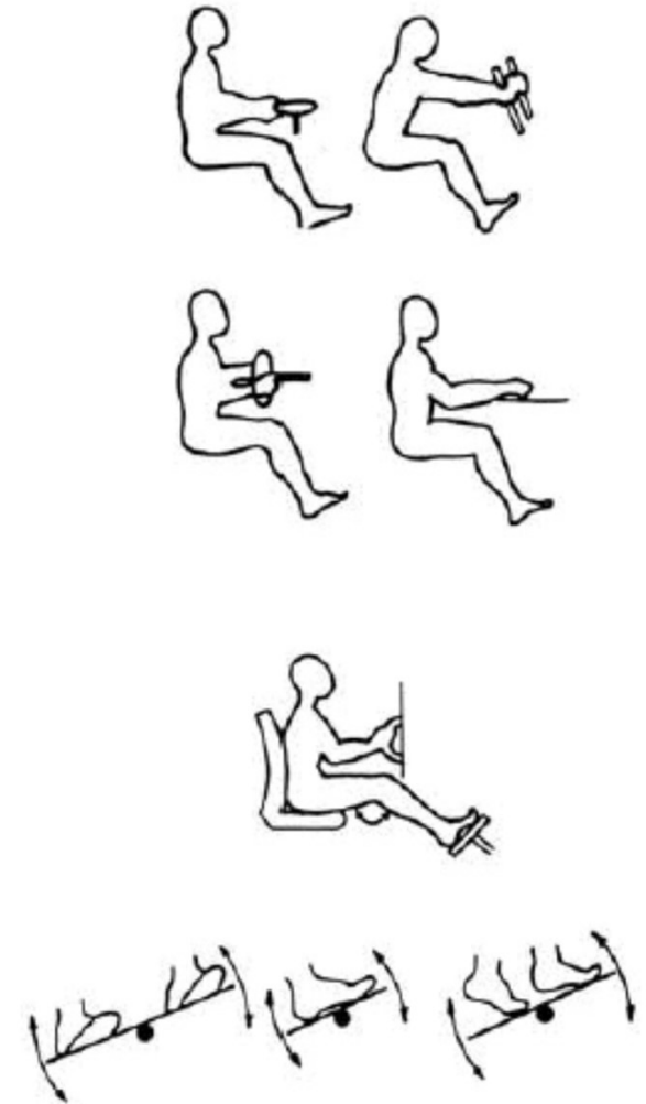
Fig. 11.2 (a) Use of hand controls and (b) Use of pedals (stable foot rest required).
