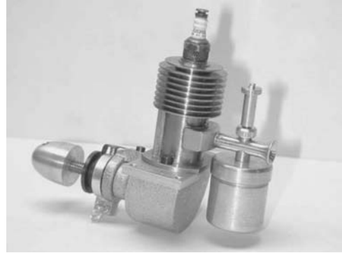
Figure 1.17 Air cooling of model airplane engine. (Courtesy R. Schroeder.)
