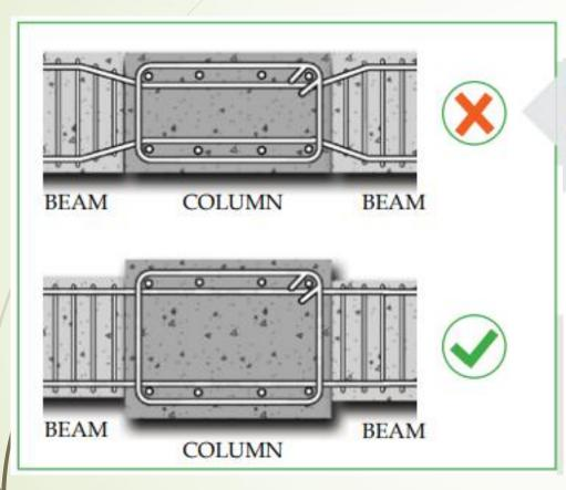
Beam bars bent in joint region overstress the core concrete adjoining the bends
