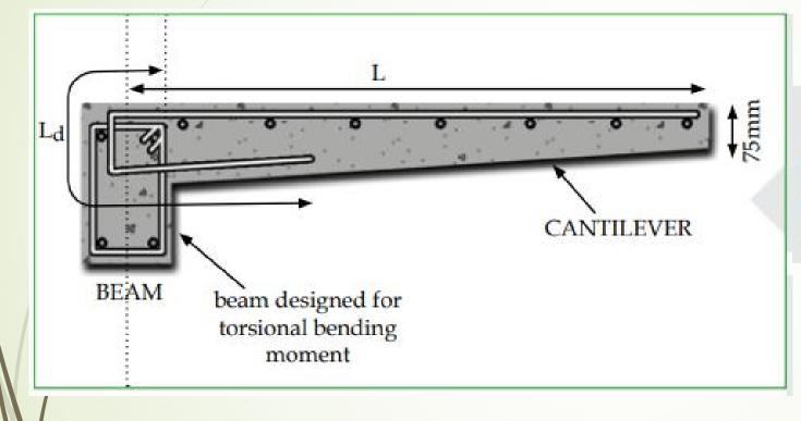
Detail for Sun-shade or any cantilever starting from top-edge of the support of the Beam 36
