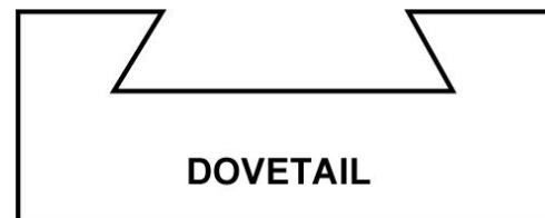
As on lathe cross slide assembly
