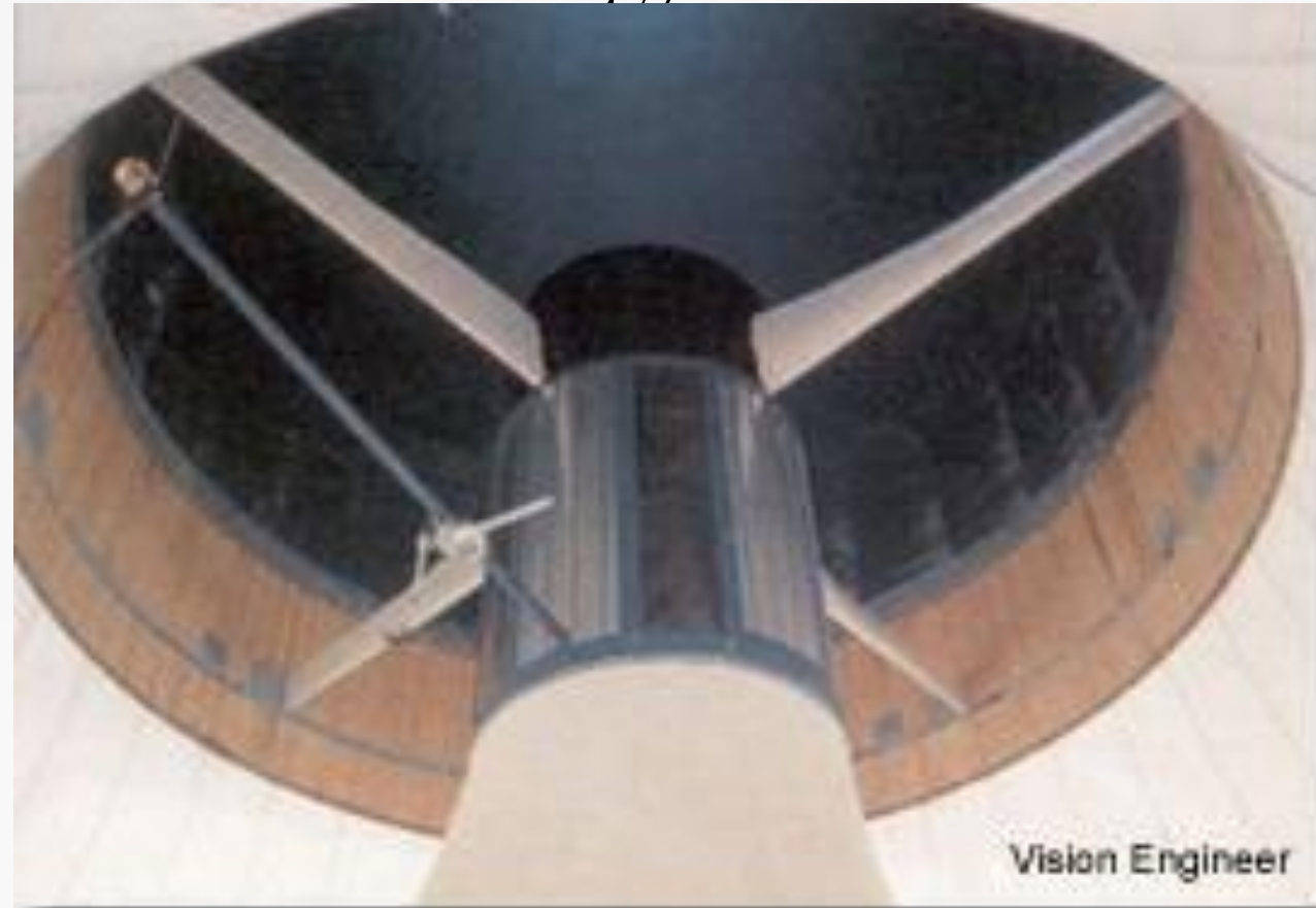
Fig Turbine for Solar Chimney Power Station
