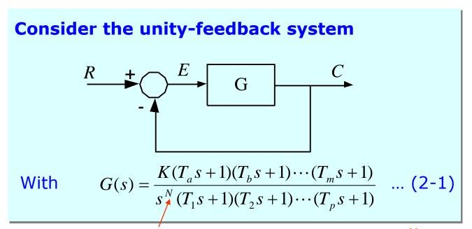
The parameter *N* associated with the term  $S^N$  in the denominator represents the "Type" of the system. <u>Example:</u> Type 0 if N=0, Type 1 if N=1 and so on.
