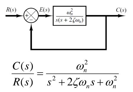
Here,  $\zeta$  and  $\omega_{\text{n}}$  are damping ratio and natural frequency of the system respectively
