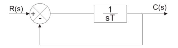
Test signal is Unit step function, R(s)=1/s
