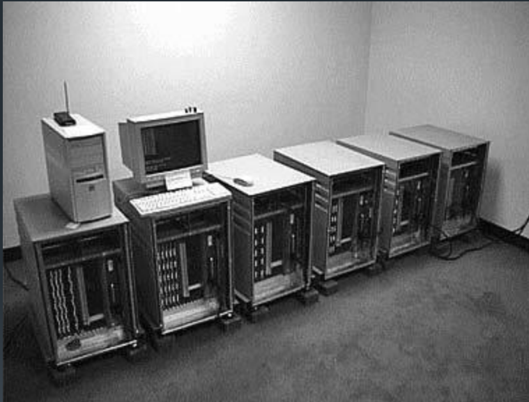
Deep Crack — the hardware exhaustive key-search machine that broke DES in 1998
