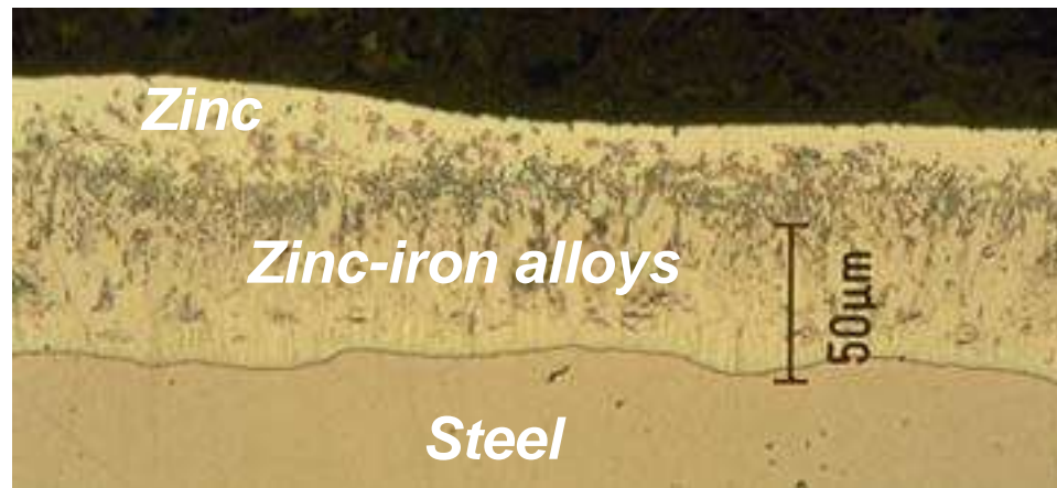
Micrograph of hot dip galvanized coating
