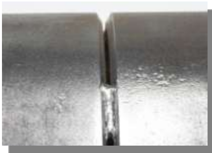
Steel Pipe – Tack Welded
