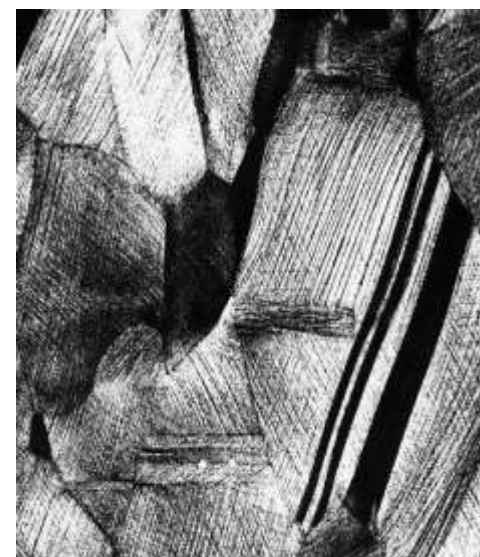
Cold Worked grains. Not annealed.
