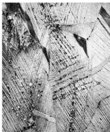
Initial recrystallization after 3 seconds @ 580°C
