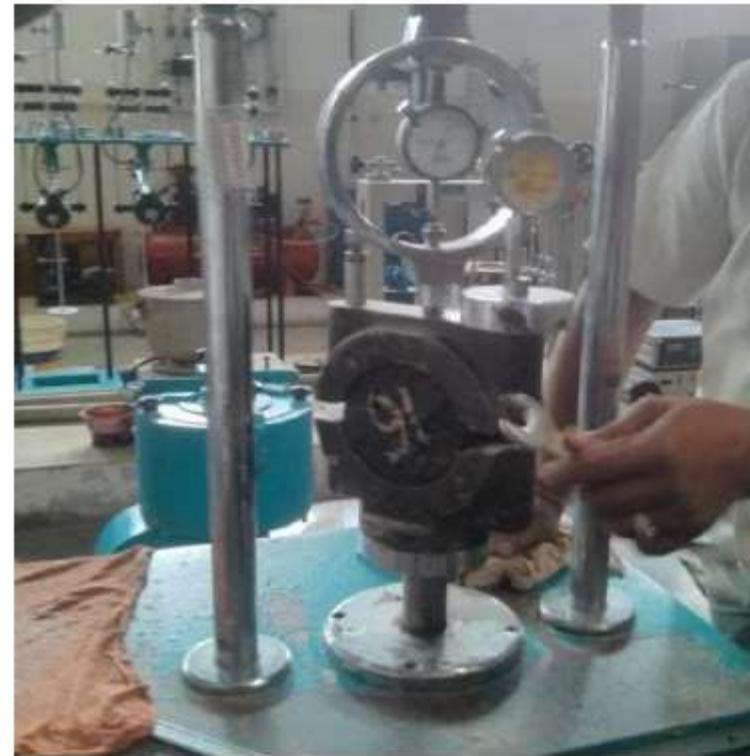
Performing marshal stability test.
