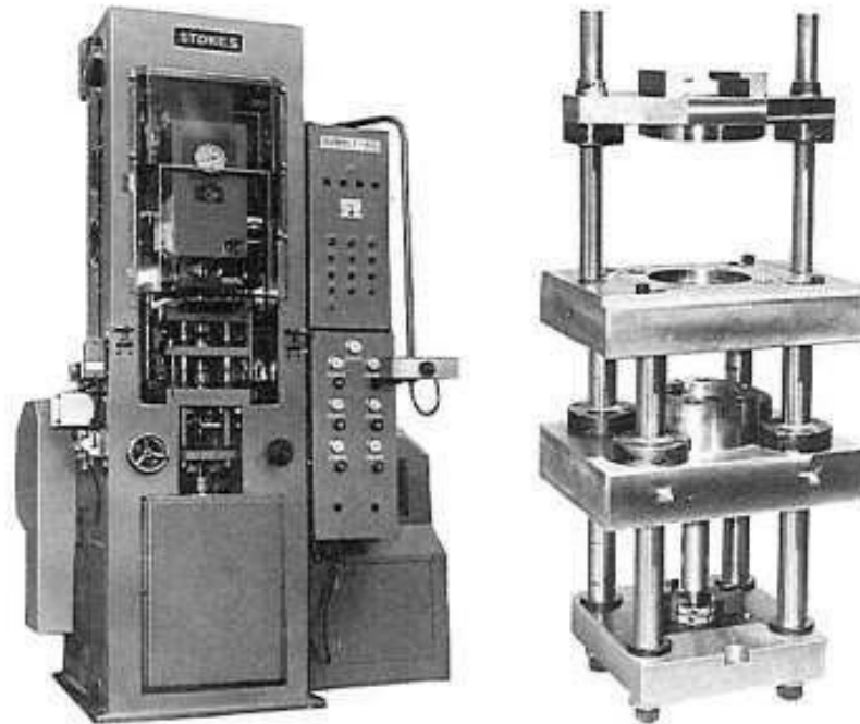
Typical press for the compaction of metallic powders. The removable die set (right) allows the machine to be producing parts with one die set while another is being fitted to produce a second part
