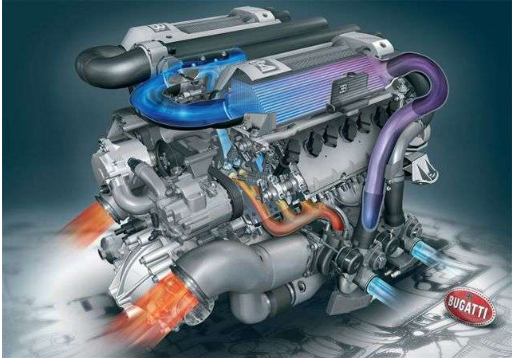
The Bugatti-Veyron engine producing 1001 hp at 6000 rev/min, 8L V-16 engine
