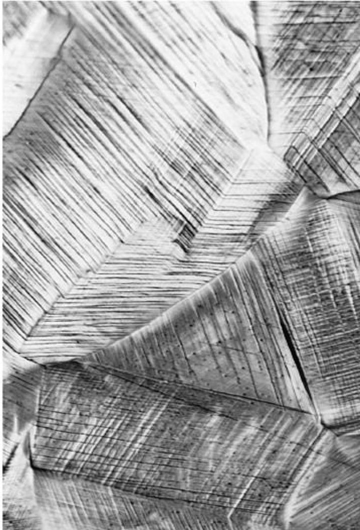
**FIGURE 7.10** Slip lines on the surface of a polycrystalline specimen of copper that was polished and subsequently deformed. 173 $\times$ . [Photomicrograph courtesy of C. Brady, National Bureau of Standards (now the National Institute of Standards and Technology, Gaithersburg, MD.)]
