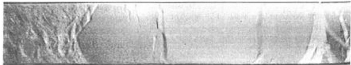
Figure 12.18. Lüder's bands on a low carbon steel tensile specimen. From S. Kalpakjian, *Mechanical Processing of Materials*, Van Nostrand, 1967, p. 194. Courtesy of J. F. Butler, Jones and Laughlin Steel Corp.
