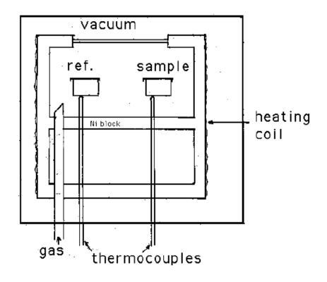
Fig. 1: Schematic illustration of a DTA cell.
