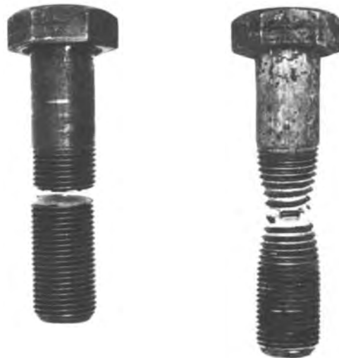
Fig. 1 Brittle versus ductile fracture in two 1038 steel bolts deliberately heat treated to have greatly different properties when pulled in tension. The brittle bolt (left) was water quenched with a hardness of 47 HRC, but had no obvious deformation. The ductile bolt (right) was annealed to a hardness of 95 HRB (equivalent to 15 HRC) and shows tremendous permanent deformation.
