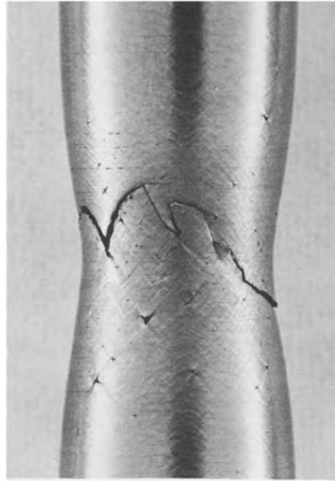
Fig. 3 Low-carbon cast steel test specimen emphasizing 45° shear aspect of tensile fracture of a ductile metal. Diagonal ridges are “Lüders lines” or “stretcher strains”; porosity in steel shows many localized fractures.
