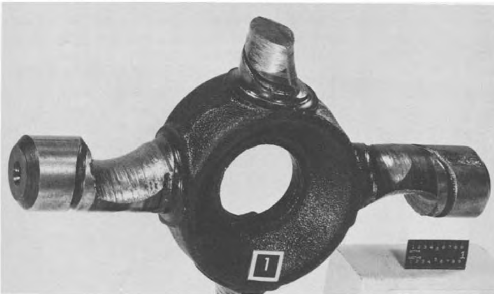
Fig. 10 Destructive adhesive wear of a differential cross following fracture of one severely worn trunnion. This vehicle was operated primarily in forward speeds; consequently only the forward-drive side was damaged severely by the rotation of differential pinions on the trunnions. The lubricant was inadequate for this application. The differential cross, or spider, and the differential pinions were made of carburized and hardened steel
