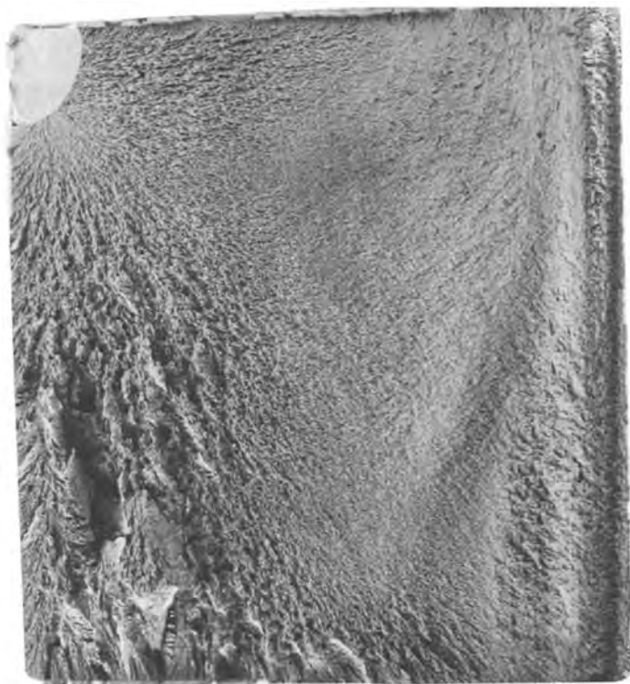
Fig. 9(a) Fracture surface of a large ( \sim 5\frac{3}{4} \times 6 in.) equalizer bar made from D6B steel heat treated to a hardness of 45–47 HRC. This bar, which supports the front end of a large crawler tractor, was in service for about 200 h and was then returned to the laboratory, where it was flexed in high-stress, low-cycle fatigue, fracturing at 60,000 cycles. Note that the fatigue-crack zone at upper left has a very fine texture, the result of continual testing. Note also the radial, fan-like ridges emanating from the fracture origin and the very small shear lips around the periphery of the brittle fracture. This fracture of a very large, high-strength part released a large amount of energy in a very short time.
