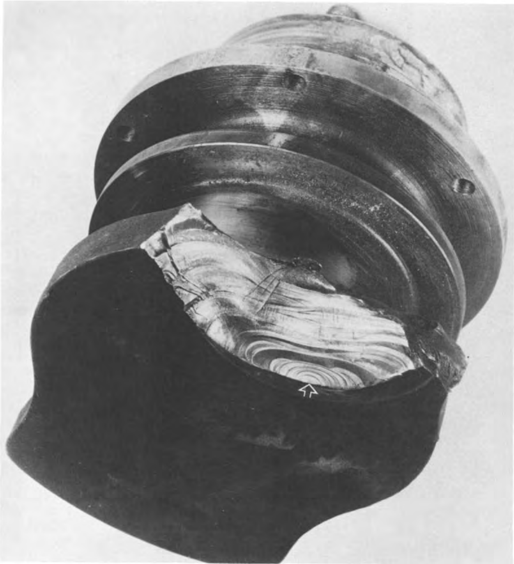
Fig. 25 Bending fatigue fracture through the cheek of a diesel engine crankshaft. The very prominent steps and beachmarks were the result of severe overloading during starting and clutching with a very aggressive friction material in the clutch. Though this was a laboratory test, it was not operated continuously and thus more closely resembles fracture from actual vehicle service.
