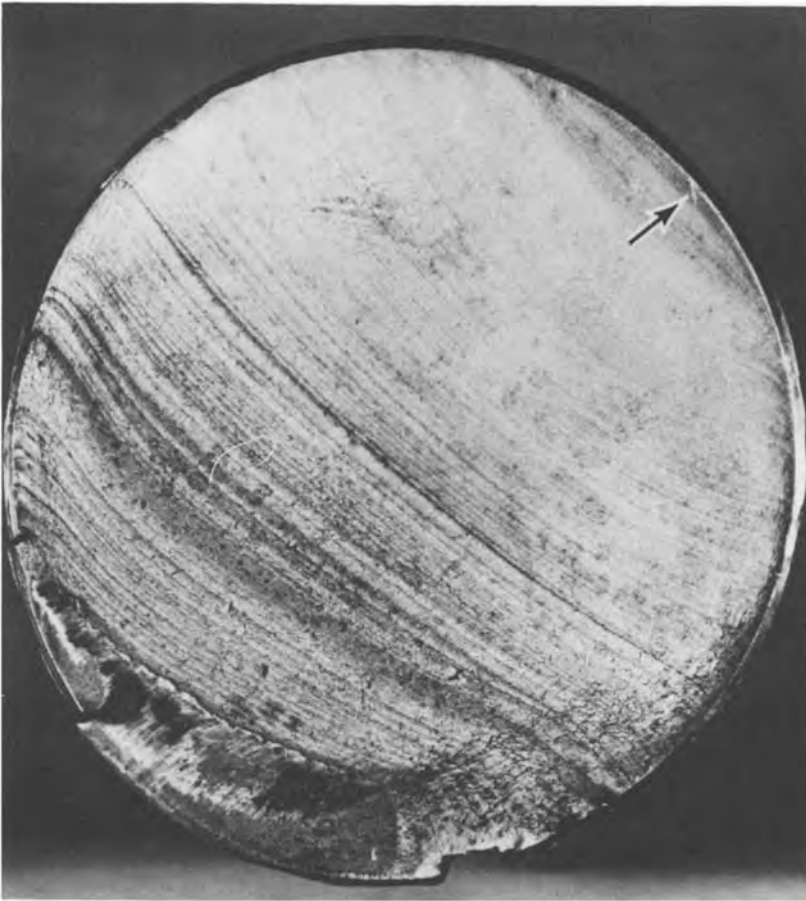
Fig. 17 Large axle shaft of medium-carbon steel with fatigue fracture across most of the cross section before final rupture. Note smooth origin region (arrow) and gradually coarsening fracture surface as the fatigue crack progressed. Note that there was a thread groove running around the periphery and that the fracture origin is in the root of the thread. However, the nominal stress was quite low because the part was still intact and operating even though the fatigue crack had gone nearly all the way through the section. This indicates that only a slight improvement in the thread groove would be necessary to prevent this type of long-term fracture.
