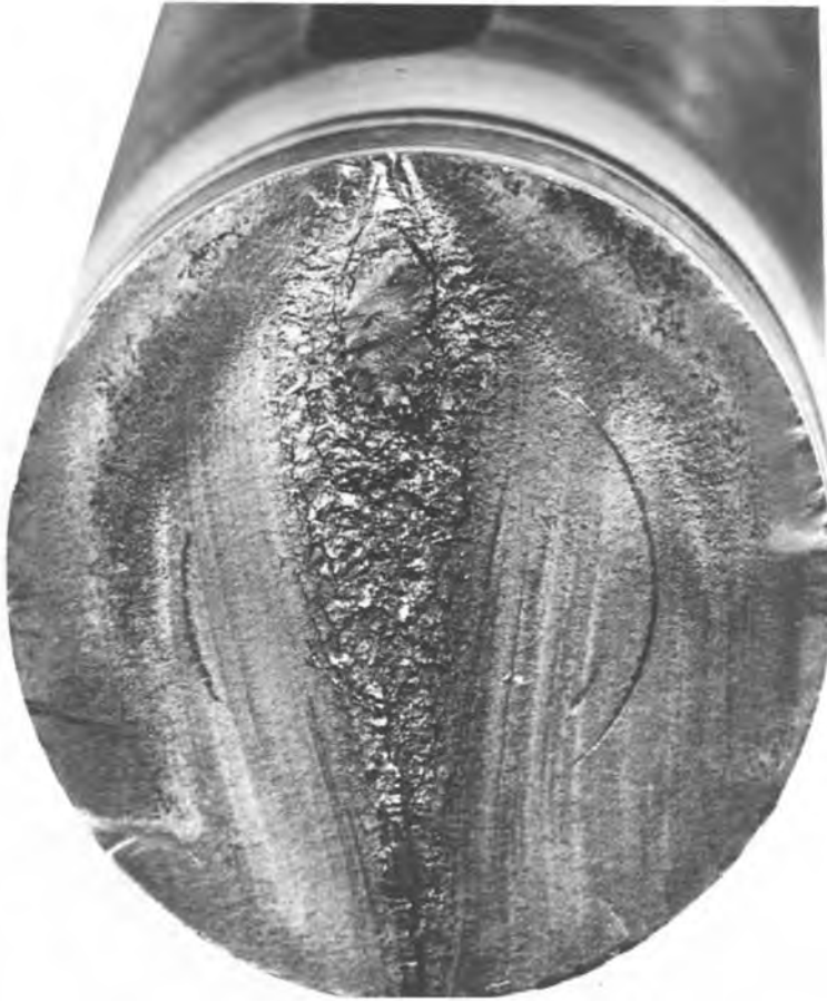
Fig. 19 Reversed bending fatigue of a 1.6 in. diam shaft of 1046 steel with a hardness of approximately 30 HRC. Note the symmetrical fatigue pattern of beachmarks on each side, with the final rupture on the diameter. This indicates that each side of the shaft was subjected to the same maximum stress and to the same number of load applications. The C-shaped marks are postfracture damage.
