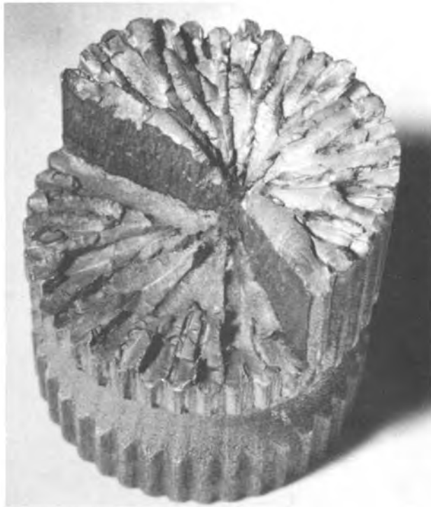
Fig. 31 A "starry" spline fracture similar to that in Fig. 30 due to reversed torsional fatigue on a 1\frac{1}{2} in. diam spline. Torsional fatigue has caused many of the surrounded segments to fall out of the shaft. Note that the longitudinal cracks penetrated nearly to the center of the shaft. This part is made from low-carbon alloy steel with a hardness of 24 HRC in the shaft area.
