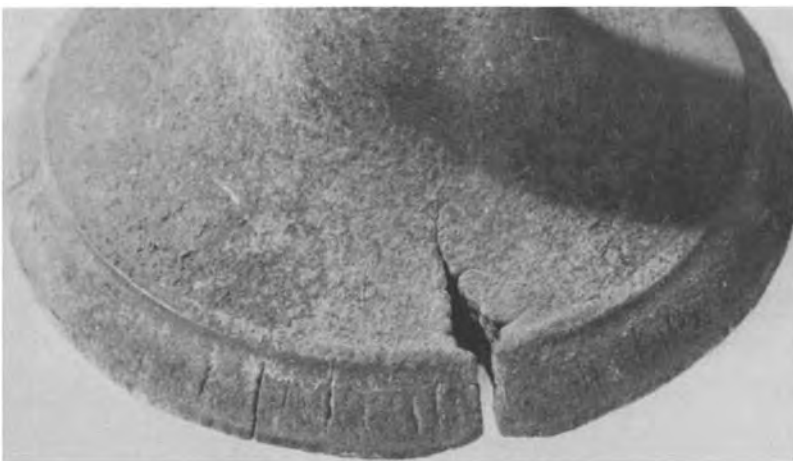
Fig. 7 Thermal fatigue crack in the hard facing alloy on an exhaust valve from a heavy-duty gasoline engine. Advanced burning originated from the large crack. Additional thermal fatigue cracks are also present on the valve face. Engine efficiency rapidly deteriorates from increasing loss of compression when very hot exhaust gases blast through the open passage (also called "blow-by"). Macrograph \sim 2\frac{1}{2}\times
