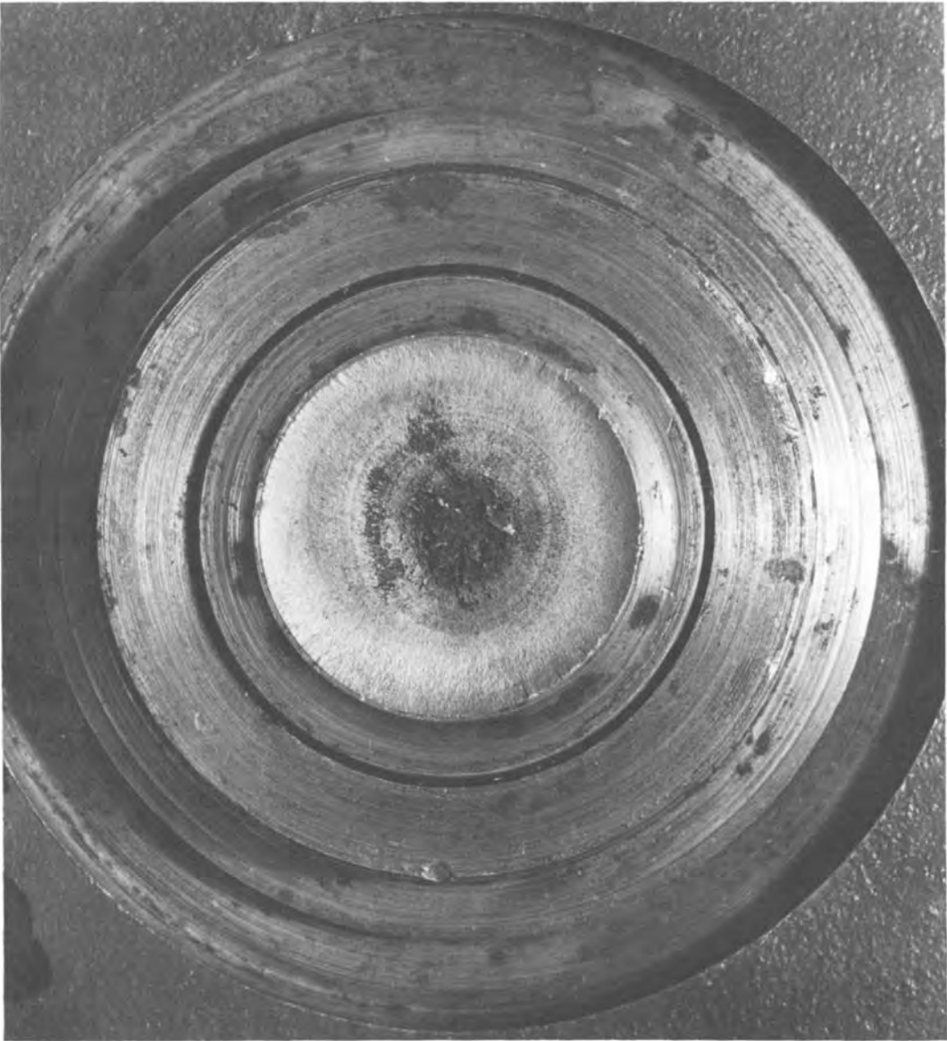
Fig. 23 Rotating bending fatigue fracture of a 2 in. diam 1035 steel shaft, hardness 143 HB. The part was designed with a large radius joining the shaft to the shoulder, but it was machined with a sharp tool mark in the fillet. Multiple-origin fatigue around the periphery proceeded uniformly into the shaft, finally fracturing with a final rupture region in the center of the shaft.
