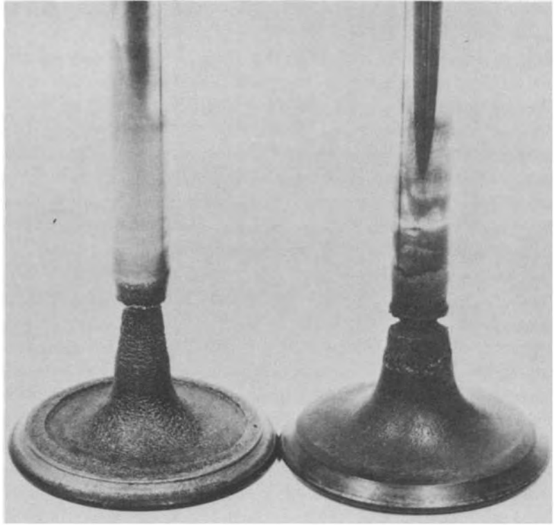
Fig. 8 Severe localized erosion-corrosion of two gasoline-fueled engine exhaust valves made from a nickel-base superalloy operating between 1400 and 1500 °F. The exhaust gas damage in the underhead radius and stem was identified as lead oxide corrosion, aggravated by bromine from the gasoline
