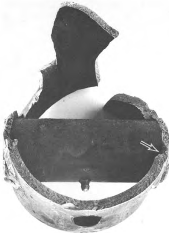
Fig. 7 Surface of a brittle fracture in a cold-drawn, stress-relieved 1035 steel axle tube. Fracture originated at a weld defect (arrow) during testing in very cold weather. Note well-defined chevron marks clockwise from the arrow pointing back toward the origin. Note also that the steel around the access hole below the grease fitting is actually necked down along the tube axis. The upper side of the tube is deformed and torn in a ductile manner.
