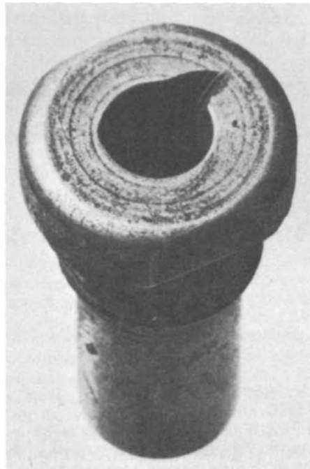
Fig. 2 Abrasive wear of a yarn eyelet made of hardened and tempered 1095 steel. Grooving was caused by a sharp change in direction of the yarn as it came out of the hole. Service life was improved by changing the eyelet material to M2 high-speed tool steel, which contains spheroidal carbides in a matrix of martensite. Service life probably could have been improved also by changing the angle of exit or by rounding the corner to make a bell-mouth hole. Source: Ref 1
