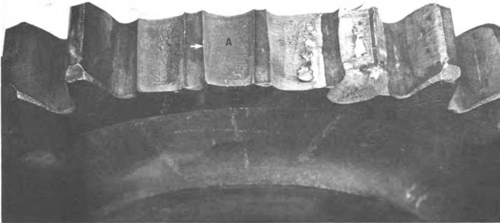
Fig. 33 Bending fatigue fractures in several teeth of an 8620 steel spur gear, carburized and hardened to 60 HRC in the case. It can be seen that tooth A fractured first, for it has the largest fatigue area, originating in the fillet on the arrow side of the tooth. Gear teeth are carefully shaped cantilever beams and can be diagnosed in this way. Fracture of the first tooth caused abnormal loading on the adjacent teeth and they also rapidly fatigued, for the mating gear did not now mesh properly with them. Considerable smashing and battering of adjacent teeth is normal after gear-tooth fracture.
