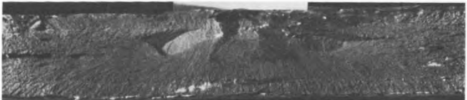
Fig. 8(b) Light fractograph of crack origin in the weld-related catastrophic fracture of the motor case shown in Fig. 8(a). 1\frac{1}{2}\times . A crack was found beneath a gas tungsten-arc repair weld on the inner surface of the case (surface at top in this fractograph) in the heat-affected zone of a longitudinal submerged-arc assembly weld. The crack was about 1.4 in. long, parallel to and 0.47 in. beneath the outer surface of the case (surface at bottom). Radial marks are visible that confirm that fracture proceeded to the left and to the right. Source: Ref 8
