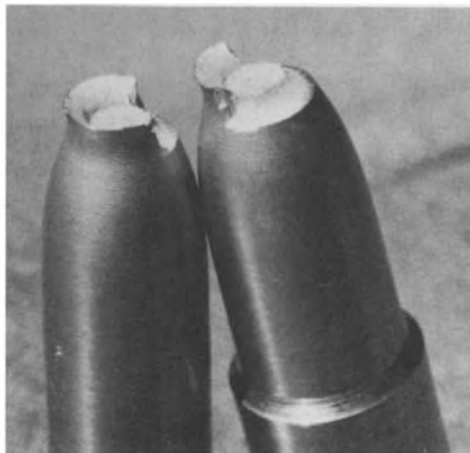
Fig. 2 Type 302 stainless steel tensile specimen with the typical cup-and-cone fracture characteristic of ductile metals fractured in tension. In this case the slant fracture at the surface of the test specimen was in both directions; in other instances it may be in only one direction, forming a perfect cup and cone.
