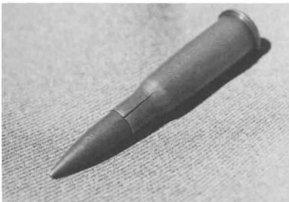
Fig. 5 Stress-corrosion crack in thin neck of a cartridge case
