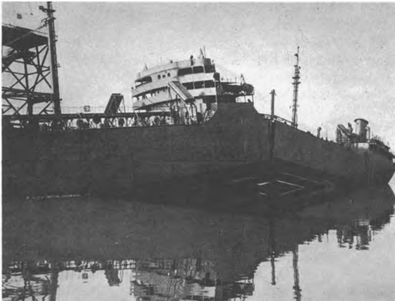
Fig. 1 New T-2 tanker, the S.S. Schenectady , which fractured in 1941 at its outfitting dock. This ship was one of 19 during World War II that had completely brittle fractures; over 200 other ships had partial brittle fractures of the hull. When tested, the fractured plates had normal ductility, as specified. Source: Ref 1
