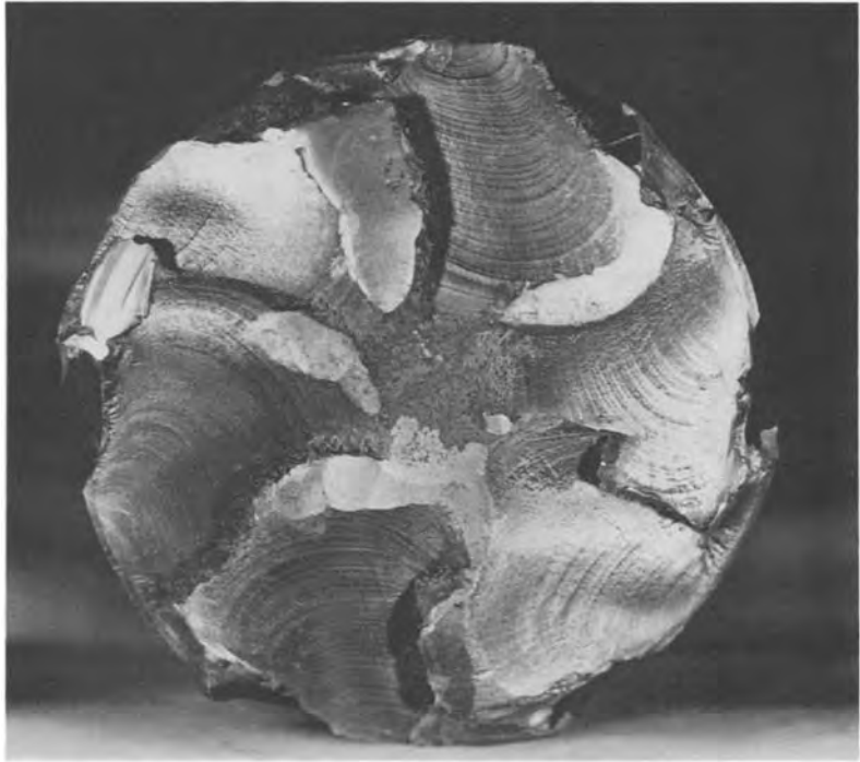
Fig. 24 Rotating bending fatigue fracture in a 4817 steel shaft, carburized and hardened to a surface hardness of 60 HRC. The fracture started in six fillet areas around the periphery, near the runouts of six grooves. The six fatigue areas penetrated separately, but uniformly, to final rupture at the center. The bright, shiny, flat areas are regions of postfracture rubbing against the opposite surface. Grinding damage in the fillet was the cause of this fracture.
