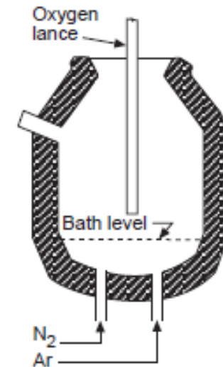
Top lance plus uncooled bottom tuyeres
