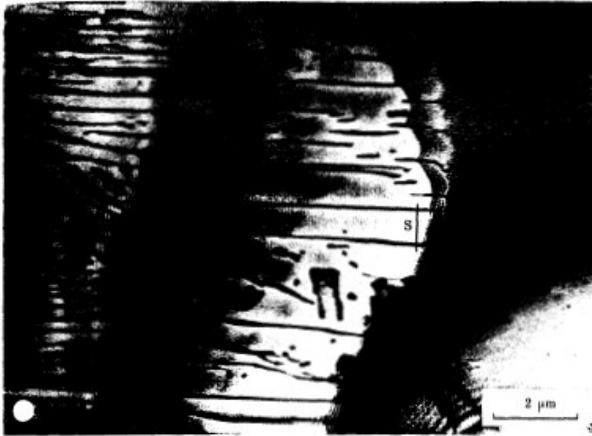
Fig. 5.53 A cell formed during ageing at two temperatures: 30 min at 220 °C followed by 30 min at 277 °C and water quenched. Note the change in interlamellar spacing caused by the change in undercooling.
