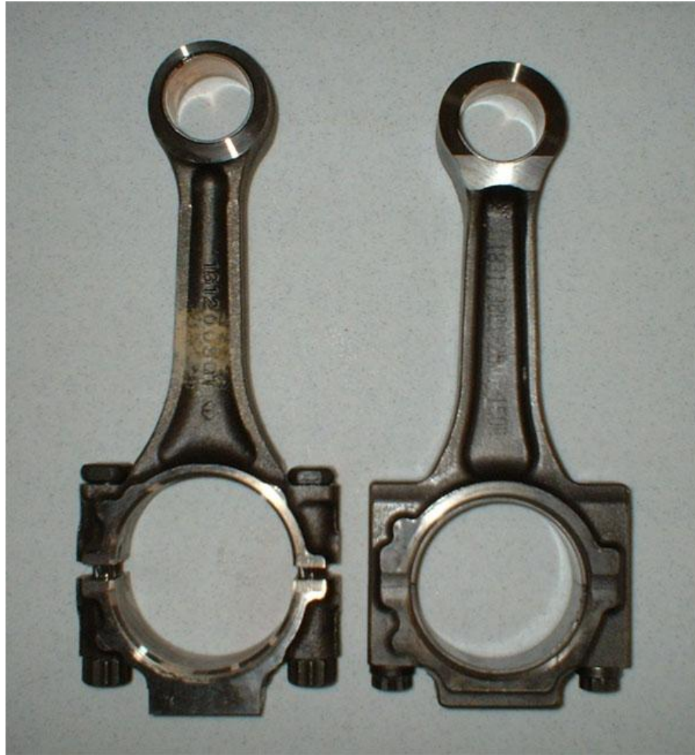
Forged on left; P/M on right
