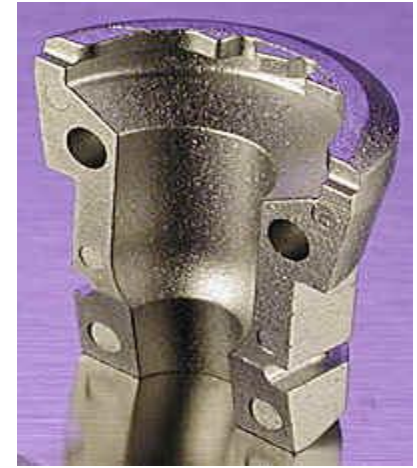
Slightly porous appearance is common
