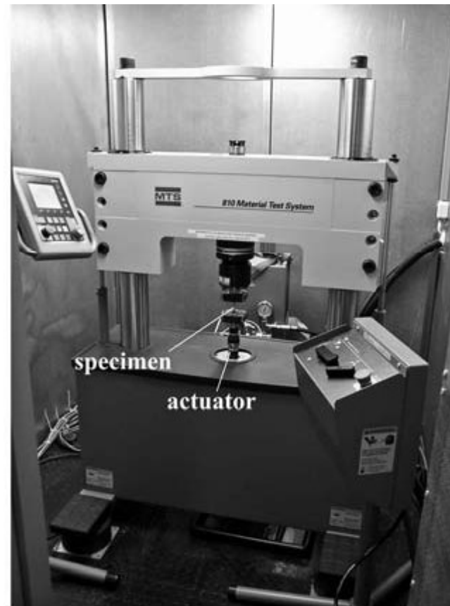
Modern servo-hydraulic push-pull testing system
