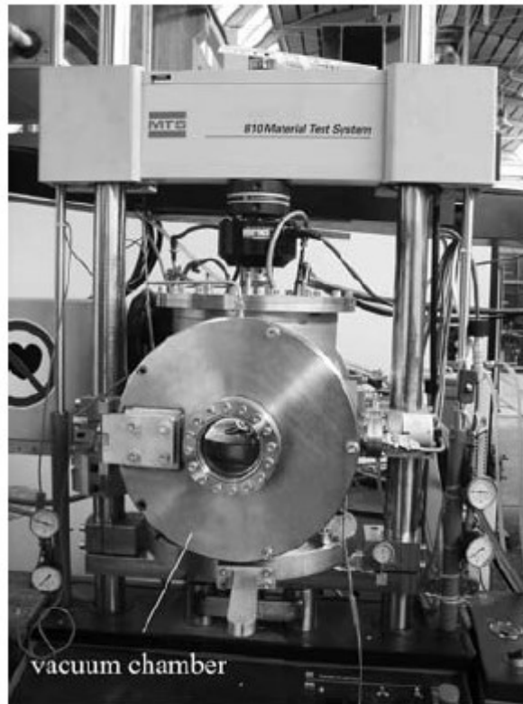
Experimental setup for high-temperature fatigue testing under vacuum or defined-atmosphere
