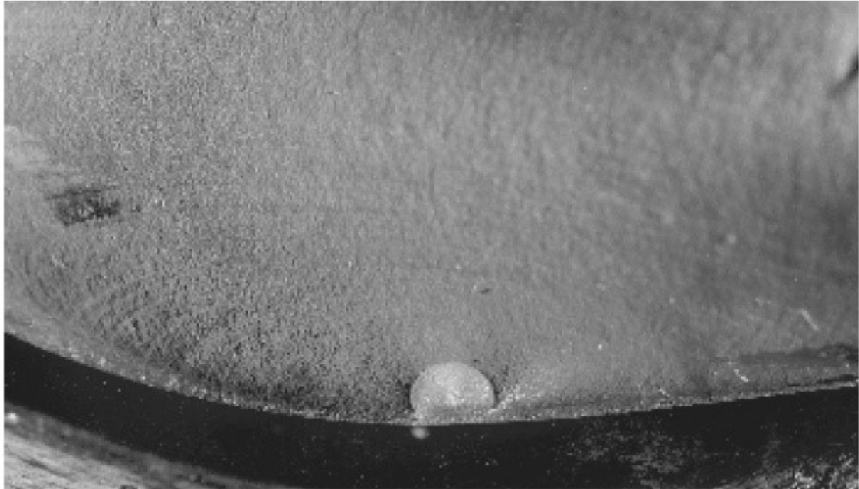
Fig.:Subsurface fatigue origin in-service failure of nitrided medium-carbon alloy steel crank pin.
