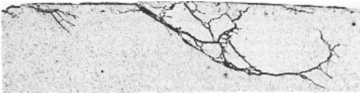
Fig.: Unetched metallographic cross section through hardened steel roller test specimen. Fatigue cracks initiate at surface
