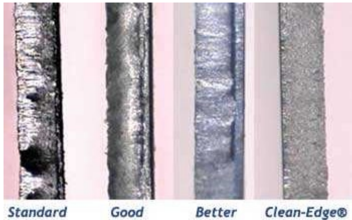
Edge condition of blanking
