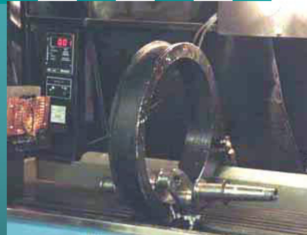
Coil on Wet Horizontal Inspection Unit
