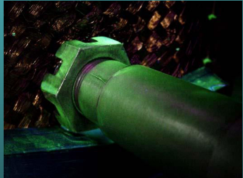
Fluorescent, Wet Particle Method
