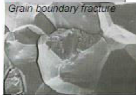
The formation of intergranular crack by grain boundary sliding
