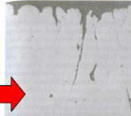
Grain boundary fracture
