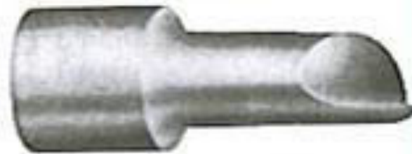
(b) Tensile (brittle) failure
