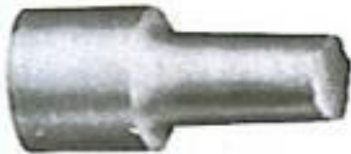
(a) Shear (ductile) failure
