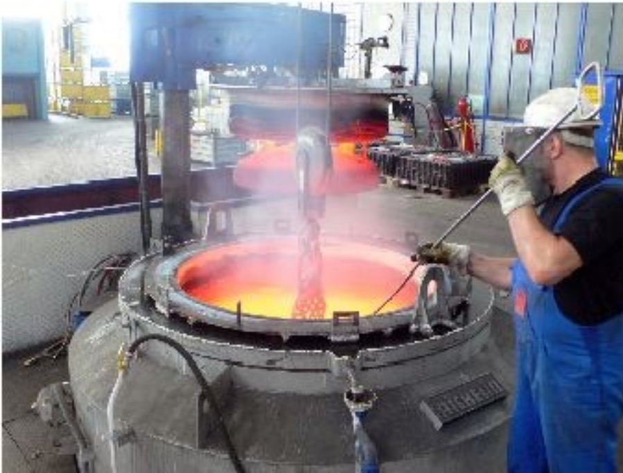
Fig. 1 : Salt bath I -austenitisation heat treatment. T = 780^{\circ}\text{C}
