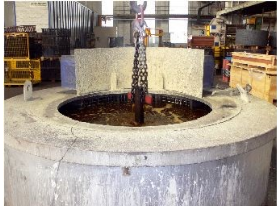
Fig. 2 : Bath II low-temperature salt-bath for isothermal treatment. T = 650^{\circ}\text{C}
