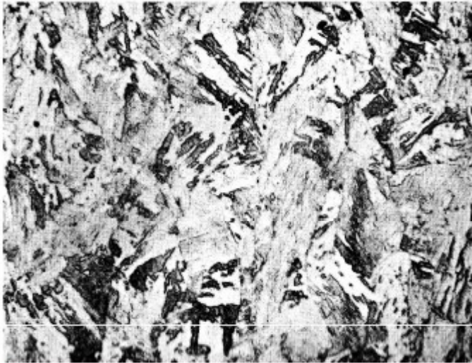
Microstructure produced by annealing 1 hr at 800°C; 100% bcc phase
