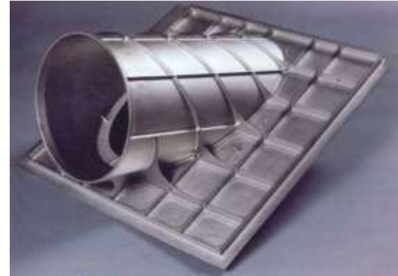
Boeing 777-APU duct- Ti-alloy
