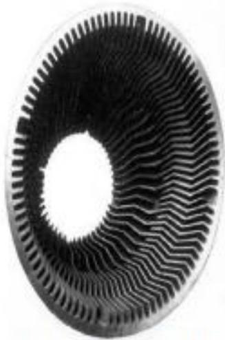
Set of steel castings for paper mill stockbreaker
