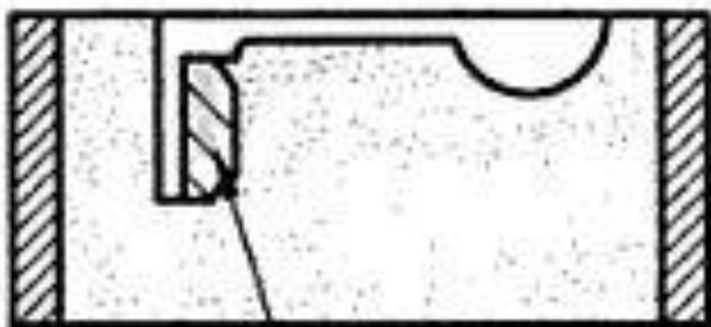
Loose piece left in the mold after pattern removal (b)
