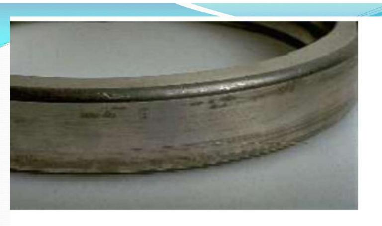
Fig. 2 Loose Fit Damage
