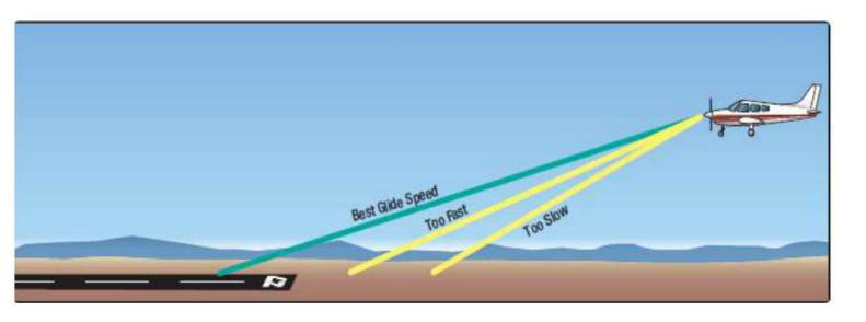
Best glide speed provides the greatest forward distance for a given loss of altitude
