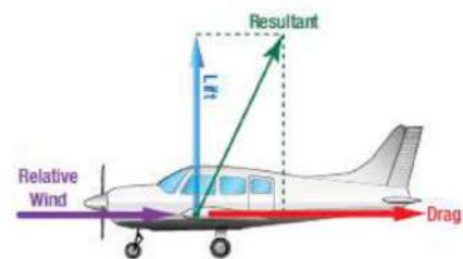
Figure 2-14. Resultant of lift and drag.
