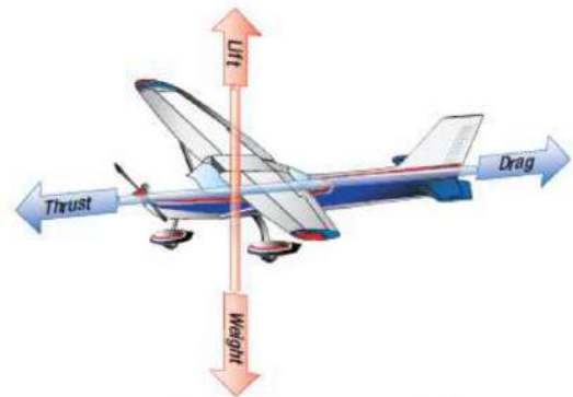
Figure 2-13. Forces in action during flight.
