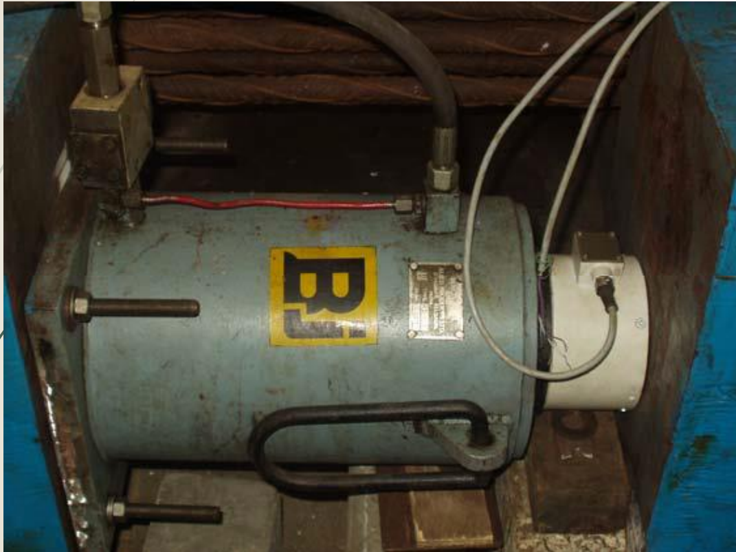
A double acting hydraulic jack with a load cell
