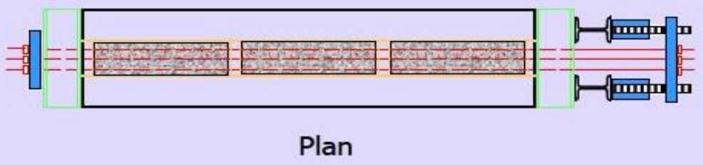
The stress bench after casting concrete
