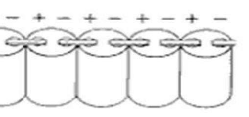
Positive terminal of one cell is connected to the negative terminal of the next, is called series connected battery.
