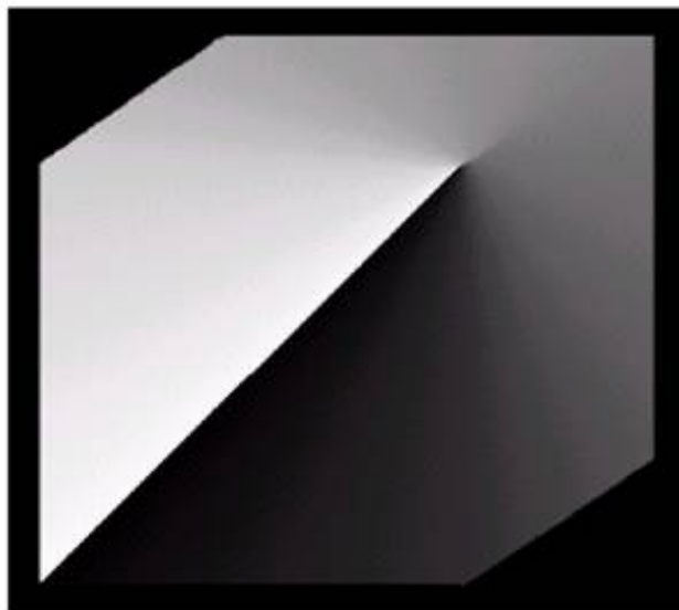
H, S, and I Components of RGB Colour Cube
