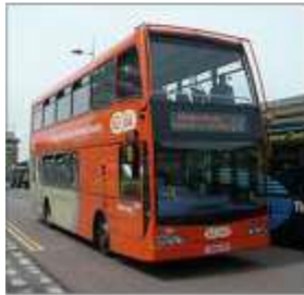
An East Lancs Olympus body with a tree protection bull-bar protecting the large upper deck front window c.coomarasamy
