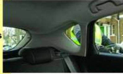
Small windows and a wide C pillar create a large blind spot in the 2009 Astra
