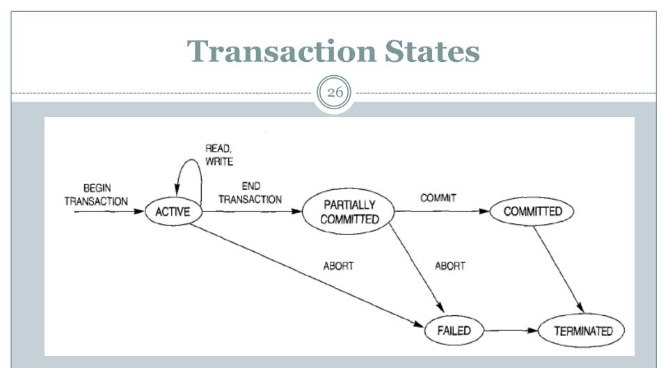
Figure shows a state transition diagram that describes how a transaction moves through its execution states.
