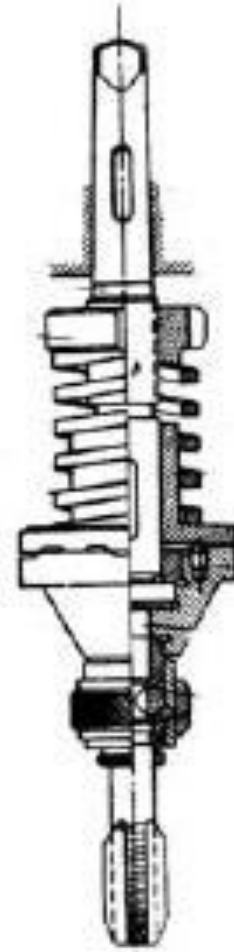
Fig. Tapping attachment for machining internal threads in drilling machines.
