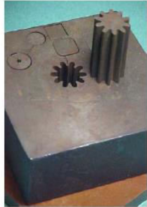
Fig. Production of teeth of external and internal spur gears by Wire-Electrodischarge machining (EDM)
