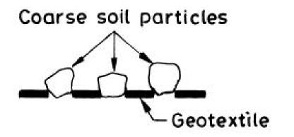
Blinding is a phenomenon similar to blocking and is used to describe the mechanism occurring when coarse particles retained by the geotextile, or geotextile fibres, intercept fine particles migrating from the soil in such a way that a low-permeable layer (often called *soil cake*) is formed very quickly at the interface with the geotextile, thereby reducing the hydraulic conductivity of the system.
