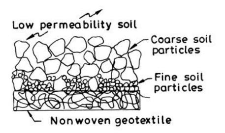
The phenomenon of accumulation of soil particles within the openings (voids) of a geotextile, thereby reducing its hydraulic conductivity, is called *clogging*. This phenomenon may result in a complete shut off of water flow through the geotextile filter.
