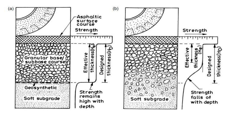
Geosynthetics, especially bitumen-impregnated geotextiles, are used to improve the paved roads, as a separator and/or a fluid barrier, by providing capillary breaks to reduce frost action in frost-susceptible soils (fine-grained soils – silts, clays, and related mixed soils).
