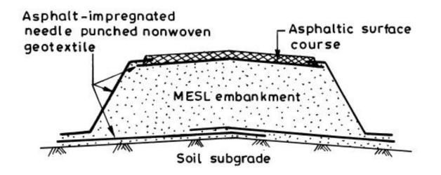
Commercially available thin-film geotextile composites are also used as moisture barriers in roadway construction to prevent or minimize moisture changes in pavement subgrades.
