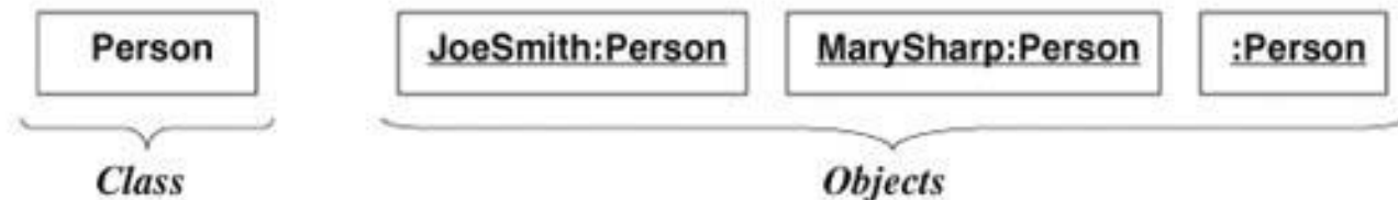
Figure 3.1 A class and objects. Objects and classes are the focus of class modeling.
