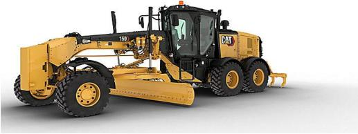
Graders are commonly used in the construction and maintenance of dirt roads and gravel roads.
