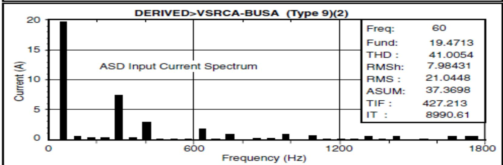
Current waveform and harmonic spectrum for an ASD input current.
