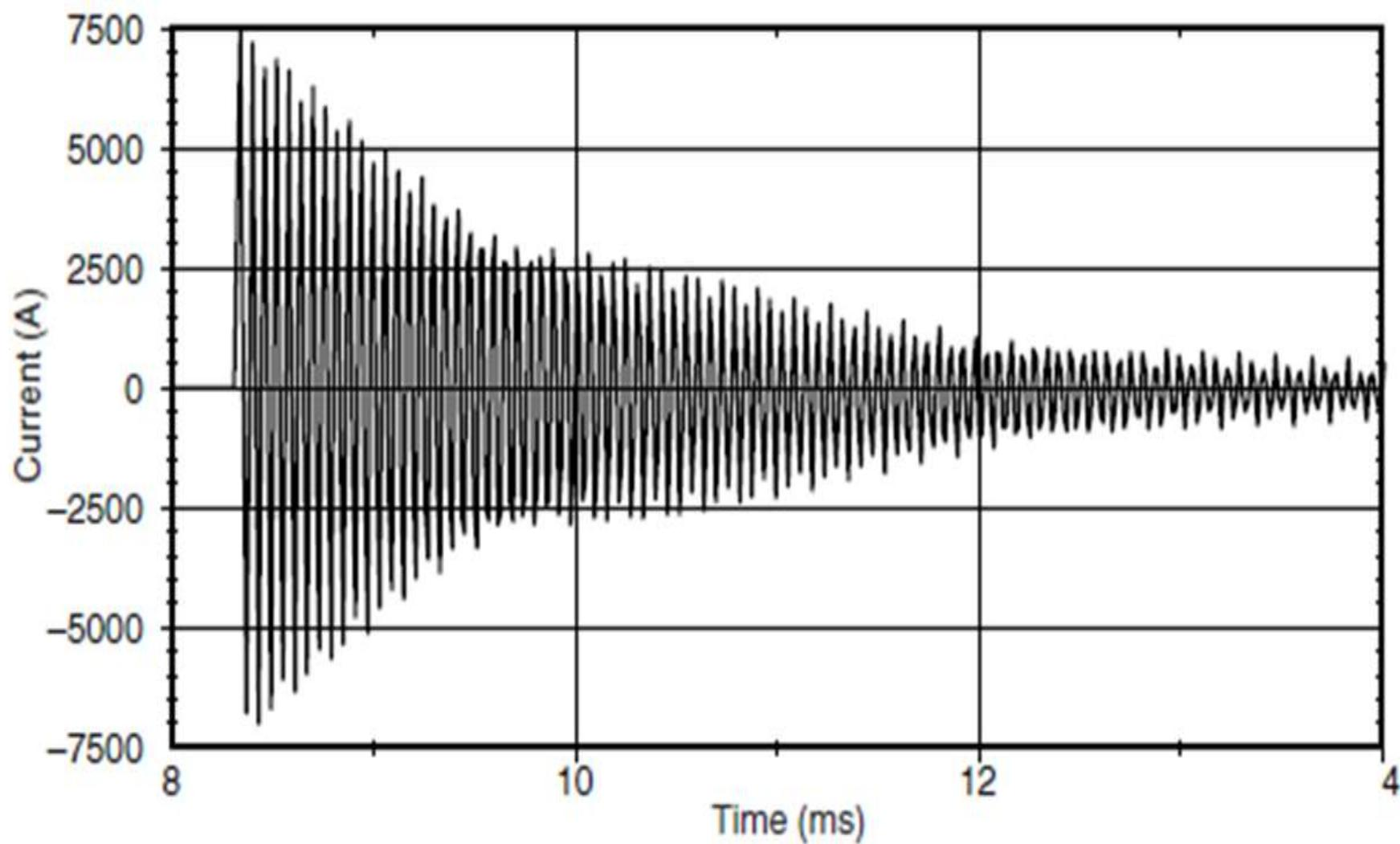
Oscillatory transient current caused by back-to-back capacitor switching.
