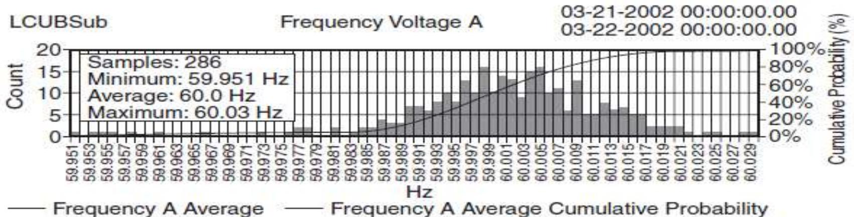
Power frequency trend and statistical distribution at 13-kV substation bus. (Courtesy of Dranetz-BMI/Electrotek Concepts.)
