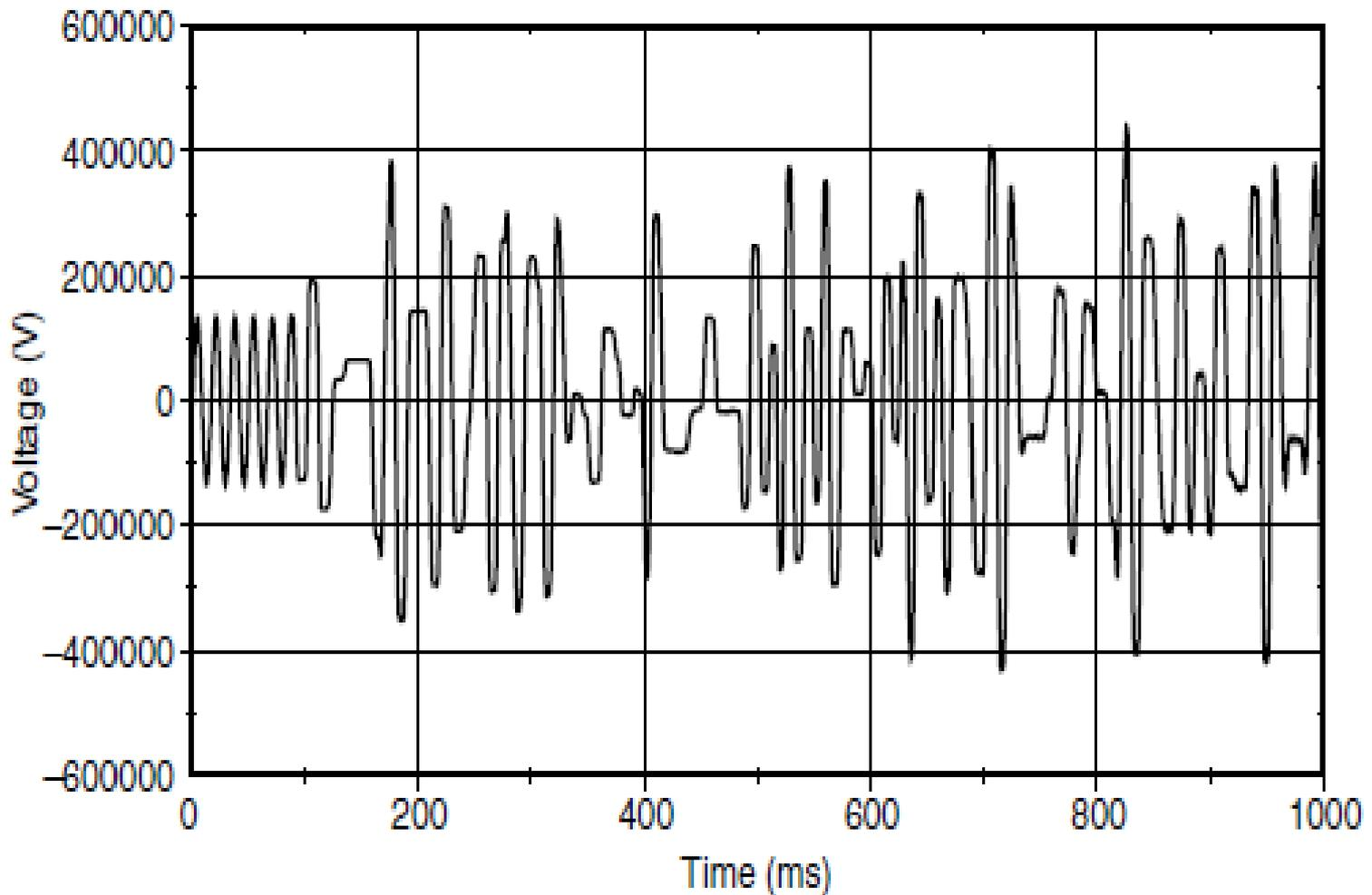
Low-frequency oscillatory transient caused by ferroresonance of an unloaded transformer.
