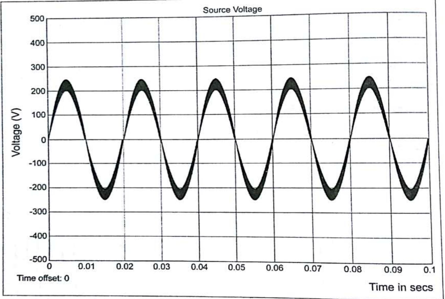
*Fig. 1.21. Voltage waveform contaminated with random white noise*
