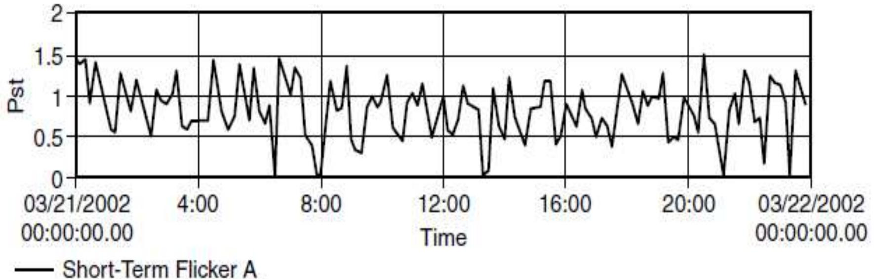
Flicker ( $P_{st}$ ) at 161-kV substation bus measured according to IEC Standard 61000-4-15. (Courtesy of Dranetz-BMI / Electrotek Concepts.)
