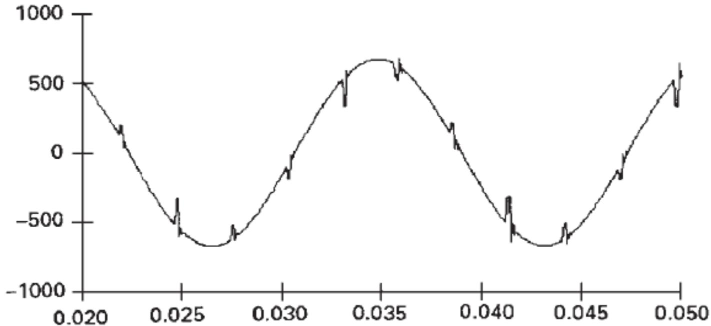
Example of voltage notching caused by a three-phase converter.
