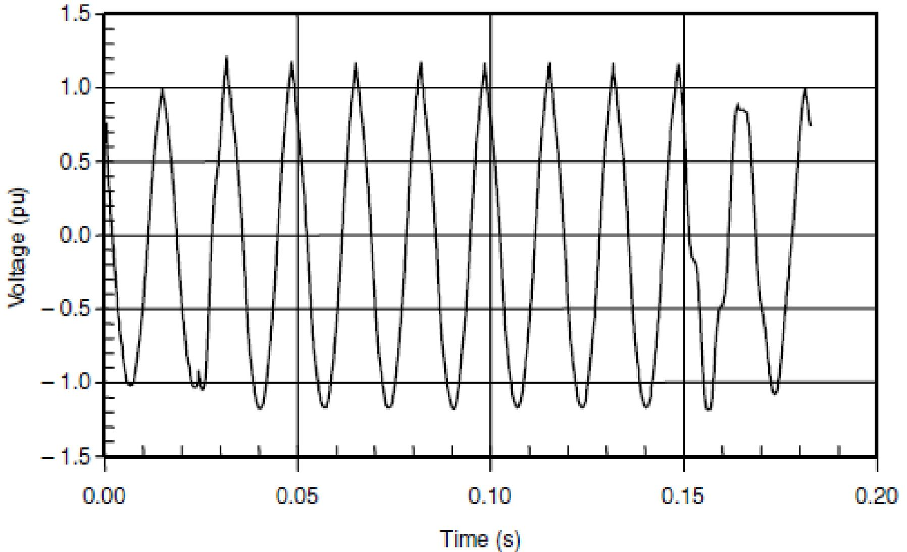
Instantaneous voltage swell caused by an SLG fault.
