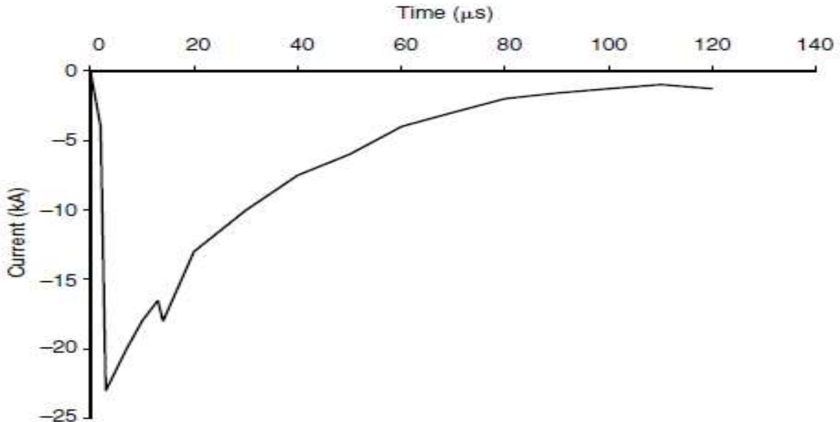
Lightning stroke current impulsive transient.
