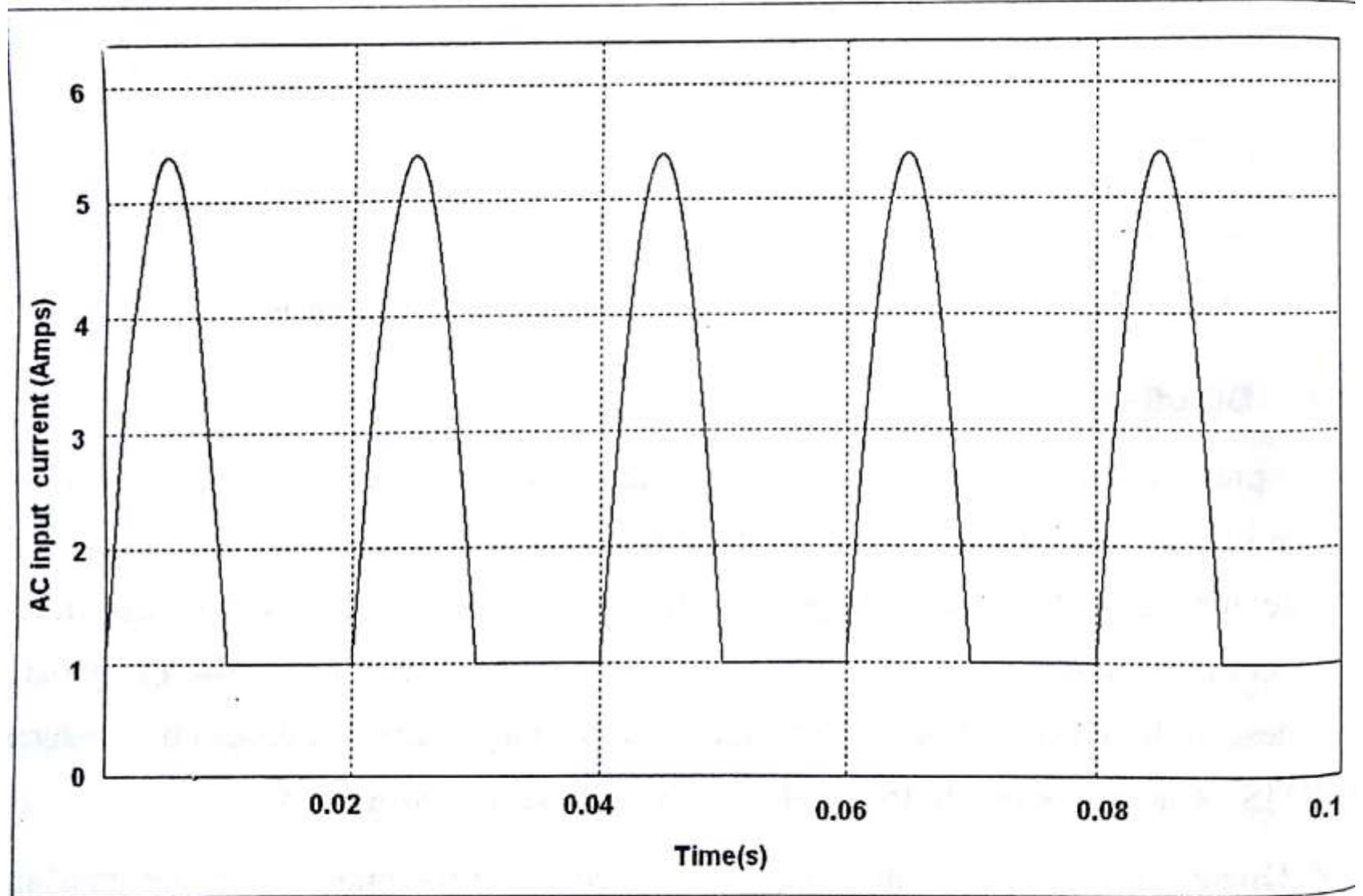
**Fig. 1.17. (b) Input current waveform consists of DC offset due to half wave rectification**
