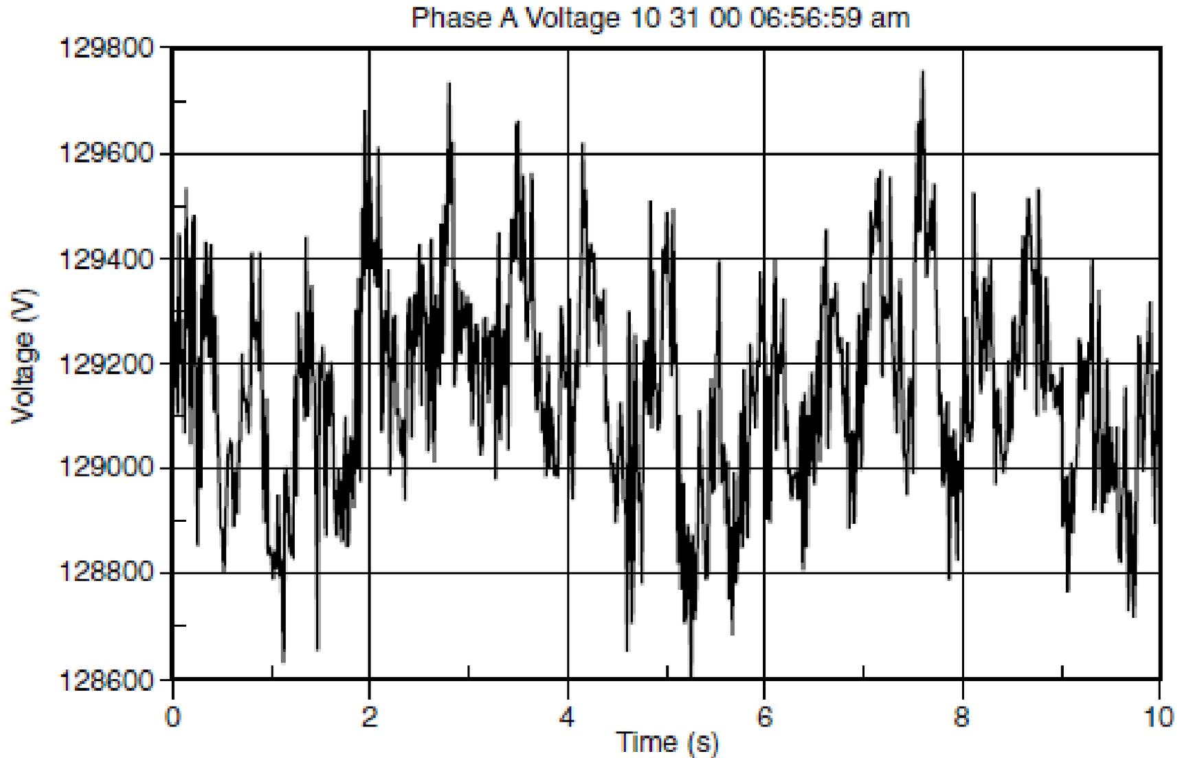
Example of voltage fluctuations caused by arc furnace operation.
