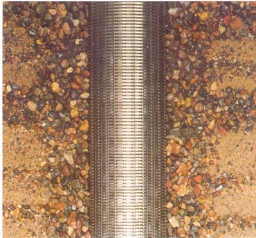
Figure 5.12 Natural development removes most particles near the well screen that are smaller than the slot openings, thereby increasing porosity and hydraulic conductivity in a zone surrounding the screen.
