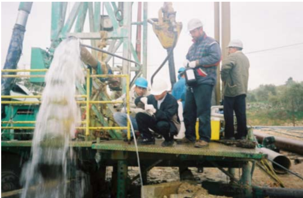
Figure 6.3 Pumping test in the field
