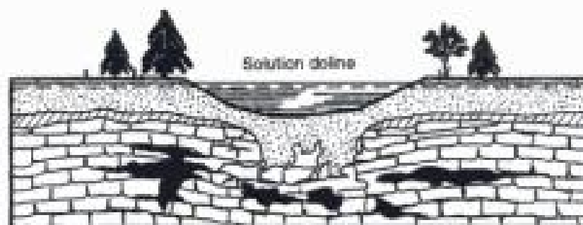
(C) Sediments from the upper layers continue to fill the openings in the limestone, causing a depression at the land surface. If water collects in the depression, a new lake is formed.
