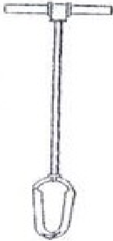
(a) Posthole or Iwan auger
